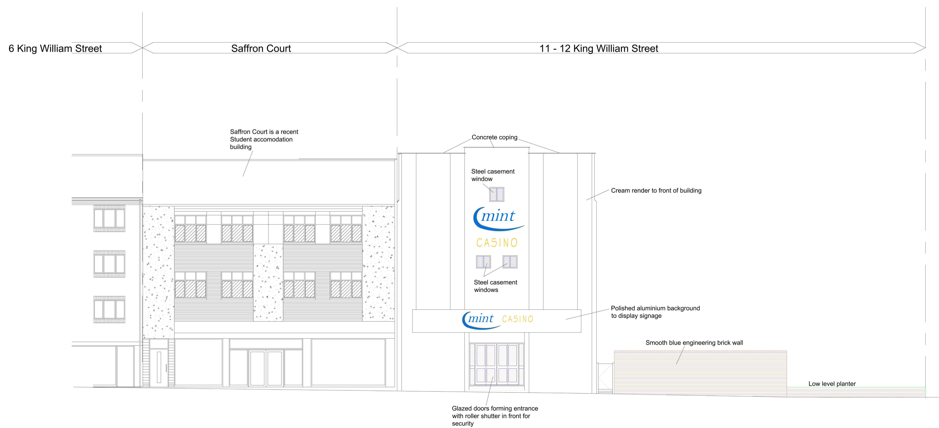
Existing Front Elevation Facing King William Street (Elevation C on Key Diagram - seen in context of street) Scale 1:100@ A1
